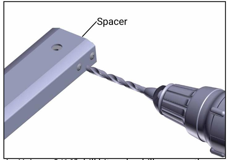
4. Using a 3/16" drill bit and a drill, remove the rivets securing the spacer. Use a hammer and punch as necessary to remove the shank of the rivets.
