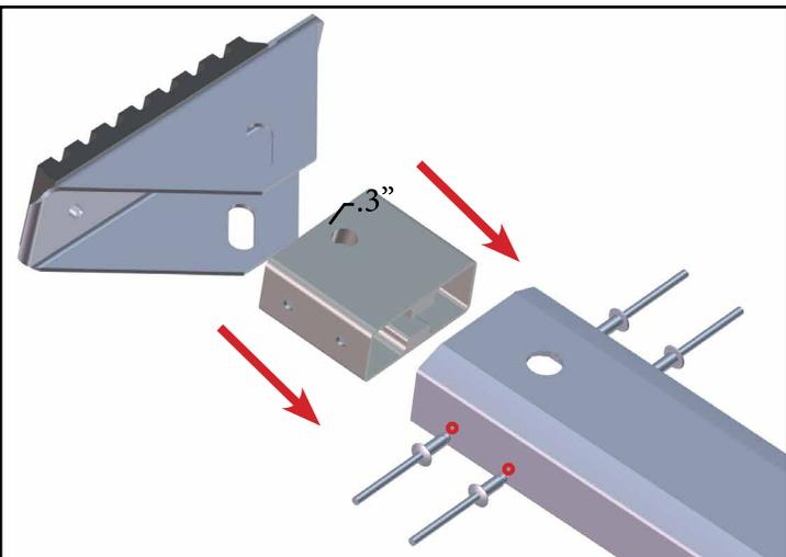
6. Insert the new spacer and secure with 4 (P/N 50129) rivets and a rivet gun.
