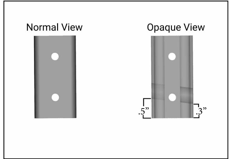
6. On one side of the spacer you have a .5" gap from the bottom to the hole, and on the other side you have a .3" gap.
