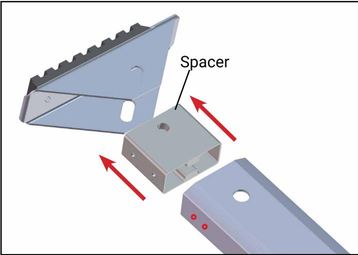
5. After removing the rivets, remove and discard the spacer.
