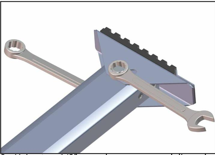
3. Using two 1/2" wrenches remove and discard the existing nut and bolt. Then remove the pick foot.
