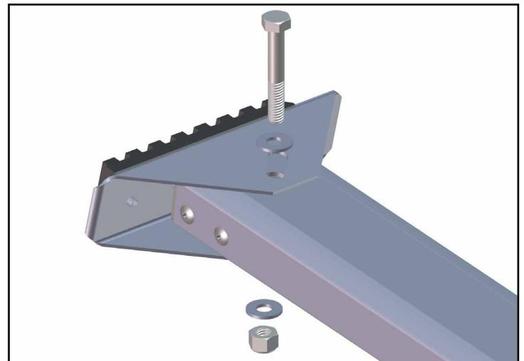
7. Once the new spacer has been secured, replace the new foot and secure with a bolt (P/N 50410), 2 washers (P/N 50411) and one nut (P/N 50412).
